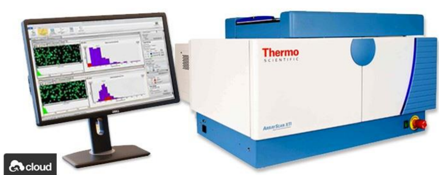
Figure 2. The Arrayscan VTI. Cells were fixed and stained and for determination of the expression of mitochondrial coded proteins as well as nuclear coded mitochondrial proteins.
