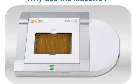
Axion's Maestro multiwell microelectrode array (MEA) platform enables high throughput evaluation of neural and cardiac activity on the benchtop, with an industry leading 768-electrodes across all plate formats.
