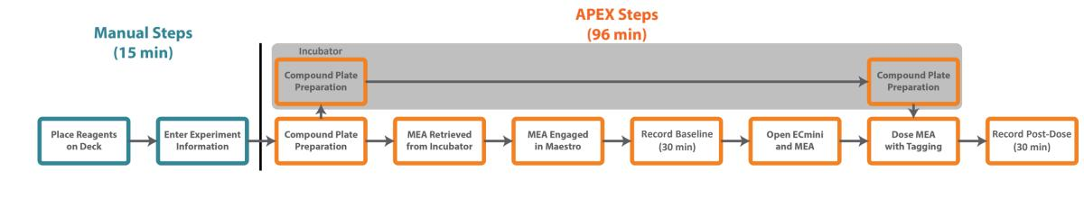
APEX offers significant efficiency gains, as user time is minimal for completing important tasks. As an example, to execute the CiPA dosing procedure, the user simply supplies the compounds at a stock concentration and enters experiment information. APEX then completes compound plate preparation, MEA plate dosing, and data acquisition, freeing the user to engage in other activities.
