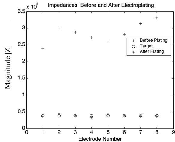
Fig. 4. Graph depicting the magnitude of impedance before and after plating for each electrode. The electrodes very nearly match their targeted impedance.
