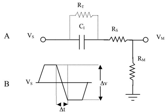
Fig.1. A) Circuit model for the microelectrode. The transfer resistance,  $R_T$ , is assumed to be infinite.  $R_S$  represents the spreading resistance,  $C_I$  is the interfacial capacitance, and  $R_M$  is the resistance of the media. B) Biphasic waveform applied at  $V_s$ .
