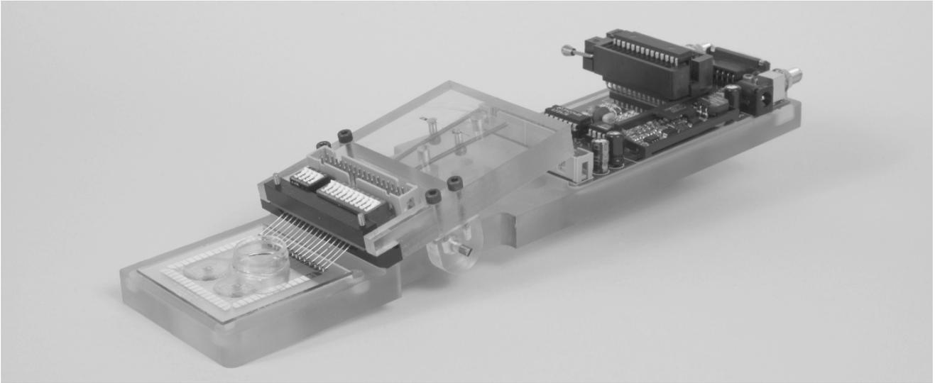
Fig. 2. Photograph of the mechanical interface and accompanying electrode impedance tuning circuitry
