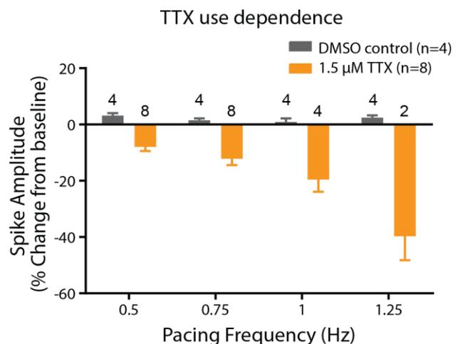
(Left) Reverse use dependence of E-4031, a hERG potassium channel blocker, revealed by pacing Pluricyte® Cardiomyocytes on the E-Stim+ Classic MEA 48 plate. (Right) Use dependence of TTX, a sodium channel blocker, revealed by pacing Pluricyte® Cardiomyocytes on the E-Stim+ Classic MEA 48 plate. (Both) Bars represent mean  $\pm$  1 standard error of the mean. Numbers above the bars indicate the number of wells successfully paced.
