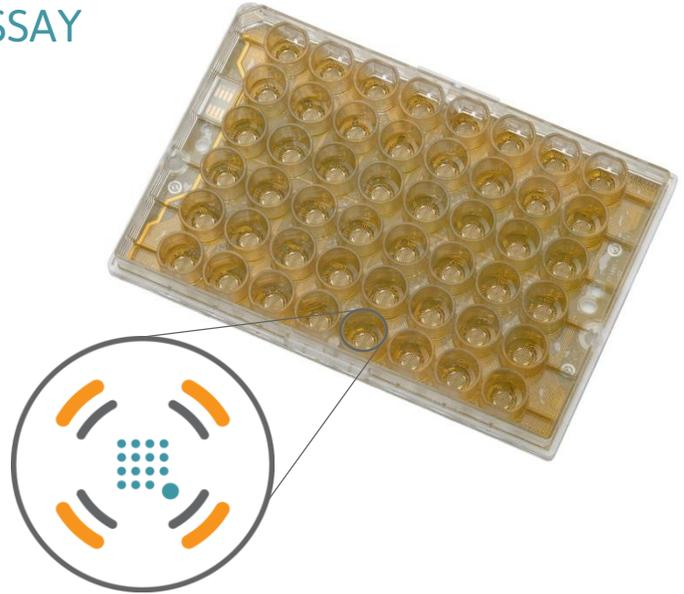
**E-Stim+ Classic MEA™ 48 plate (M768-KAP-48S).** (Inset) Schematic of well illustrating large dedicated stimulation electrode and recoding electrodes (blue), AccuSpot on-plate spotting guides (gray), and grounds (orange).
