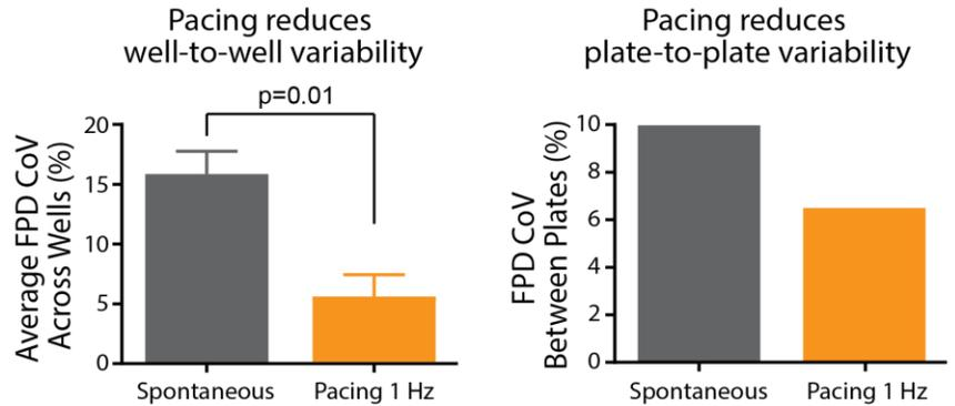
Pacing Pluricyte® Cardiomyocytes with the E-Stim+ Classic MEA plate significantly reduces well-to-well variability in field potential duration (FPD) ( $p=0.01$ ) as well as variability between plates. Variability was measured as the coefficient of variation (CoV) across wells (left) and across plates (right).
