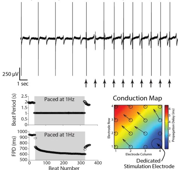
**Pacing stimuli set beat rate at 1Hz (top, arrows). Beat period and field potential duration quickly adapt (bottom left). AxIS also quantifies key parameters, such as conduction, with real-time visualization (bottom right).**
