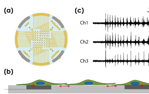
A planar arid of microelectrodes (a) interfaces with cultured neurons (b), modeling in vivo neural behavior in a dish. Electrodes detect changes in raw voltage (c) through recording of extracellular field potential.
