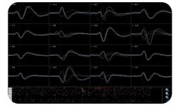
Raw voltage signals are processed in real-time to obtain extracellular action potentials from across the network via up to 64 electrodes, providing a valuable electrophysiological phenotype for applications in drug discovery, toxicological and safety screening, disease models, and stem cell characterization
