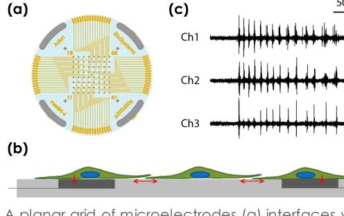
A planar grid of microelectrodes (a) interfaces with cultured neurons (b), modeling complex, human systems over an electrode array. Electrodes detect changes in raw voltage (c) through recording of extracellular field potential.
