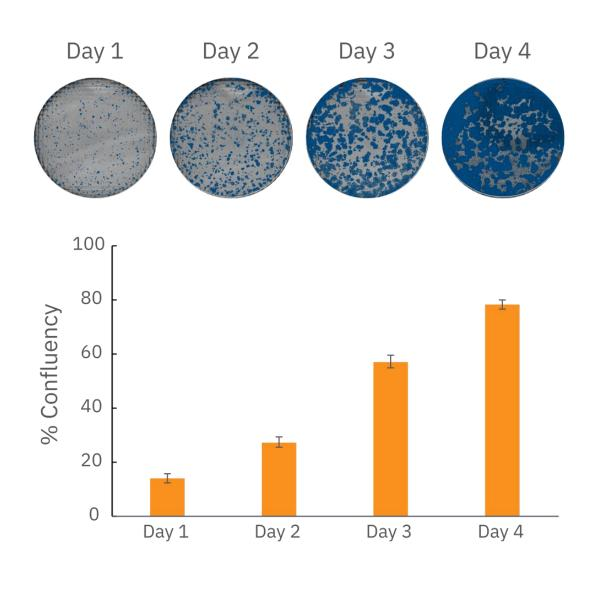
Manual inspection and estimation of culture confluence can be a time consuming and inaccurate process. Only a small fraction of a given well may be seen at once with a 2x objective, requiring the scientist to navigate across the well and mentally combine confluence estimates. The Omni full-vessel scan eliminates tedious scrolling on the microscope and provides an accurate measure of confluence.
