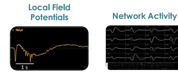
Raw voltage signals are processed in real-time to obtain extracellular field potentials from across the network, providing a valuable electrophysiological phenotype for applications in drug discovery, toxicological and safety screening, disease models, and stem cell characterization
