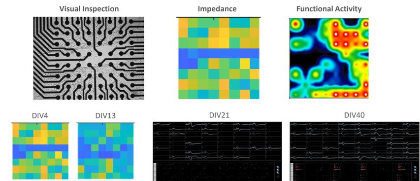
The impedance measurements illustrate how neurons and axons have migrated into the "gap" over time in culture.
