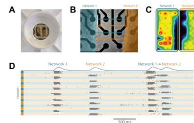
A) Two compartment silicone insert (ibidi). B) Axonal projections cross the cell-free gap within 10 days of removing the insert. C) Activity map illustrating synchronous activity between the two spatially separated networks. D) Raster plot at 17 days *in vitro* illustrating independent network activity from network 1 and network 2, followed by a whole-well network event with network 1 driving the activity in network 2.
