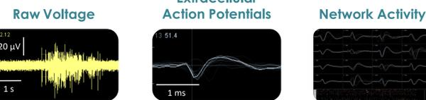
Raw voltage signals are processed in real-time to obtain extracellular action potentials from across the network, providing a valuable electrophysiological phenotype for applications in drug discovery, toxicological and safety screening, disease models, and stem cell characterization.
