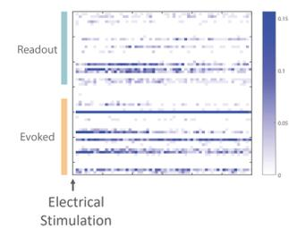
Electrical stimulation was used to evoke network activity in the "Evoked" network. Functional network activity then occurred reliably, after a propagation delay, in the "Readout" network within the well.
