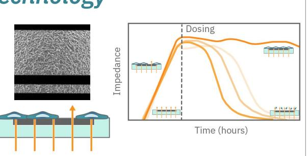
The impedance is measured from electrodes embedded in the bottom of each well. As cells cover more of the electrode, impedance increases in proportion to the number of viable cells. If a perturbation kills the attached cells, impedance decreases as the cells lyse.
