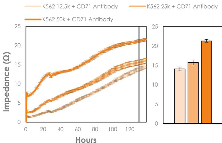
**Figure 4:** (Left) Growth curves for K562 cells seeded at 12.5k, 25k, and 50k with anti-CD71 antibody, and monitored on the Maestro Z during the attachment, spreading, and proliferation phases. (Right) At 130 hours, the higher cell density (500k) showed a larger impedance as compared to the lower cell density (12.5k).
