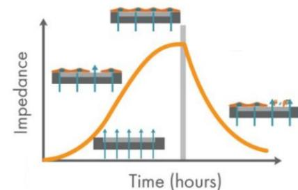
**Figure 1.** Impedance measures how much electrical signal (teal arrows) is blocked by the electrode-cell interface (right). When the electrode is uncovered, electrical signal easily passes and the impedance is low. When cells cover the electrode, less electrical signal passes and the impedance is high. When cells die or detach, the impedance decreases.
