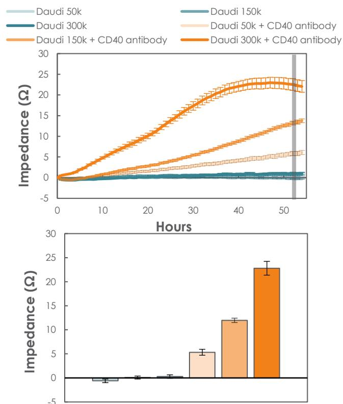
**Figure 3:** (Top) Growth curves for Daudi cells seeded at 50k, 150k, and 300k cells/well, with or without CD40 antibody, and monitored on the Maestro Z during the attachment, spreading, and proliferation phases. (Bottom) At 48 hours, the highest cell density (300k) had the largest impedance, whereas lower densities had lower impedance as they continued to proliferate. When no antibody was used, no impedance change was observed.
