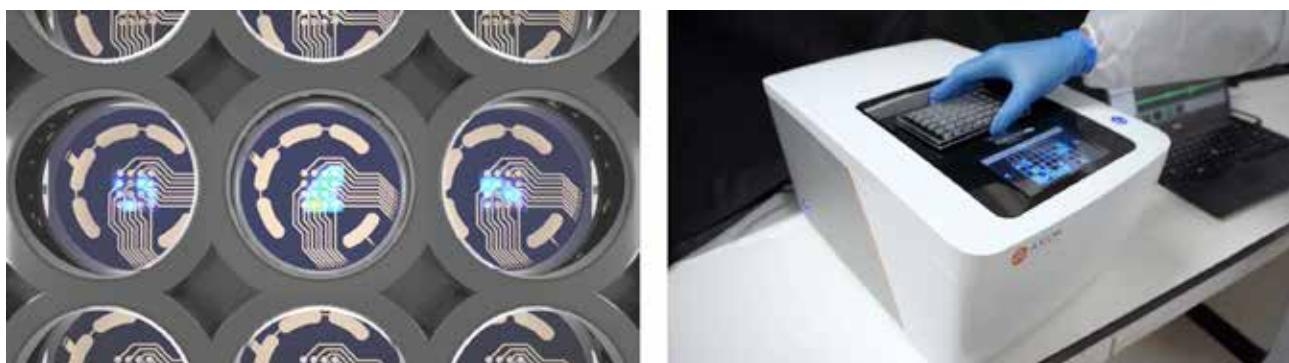
Figure 2: (Left) A Multiwell plate allow scientists to record data from 96 'brain-in-a-dish' cultures simultaneously. (Right) A scientist docking a 48-well MEA plate
