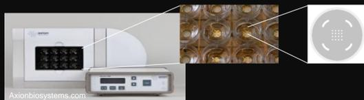
Figure 3. Axion Biosystems Maestro Multielectrode Array, 48 well plate, and 4X4 electrode grid used to collect spontaneous activity data.
