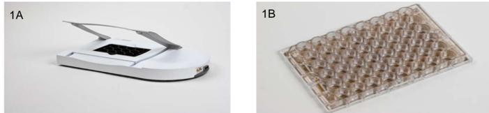
**Figure 1A.** The Maestro, Axion BioSystems. 768 recording channels with fully integrated heater and software controls. Accommodates 12, 48 and 96 well MEA plates. **Figure 1B.** 48 well configured MEA plate, Axion BioSystems. 16 microelectrodes per well, ANSI compliant, nano-textured gold electrodes with evaporation reducing lid.
