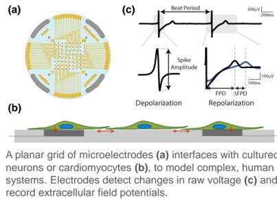
A planar grid of microelectrodes (a) interfaces with cultured neurons or cardiomyocytes (b), to model complex, human systems. Electrodes detect changes in raw voltage (c) and record extracellular field potentials.
