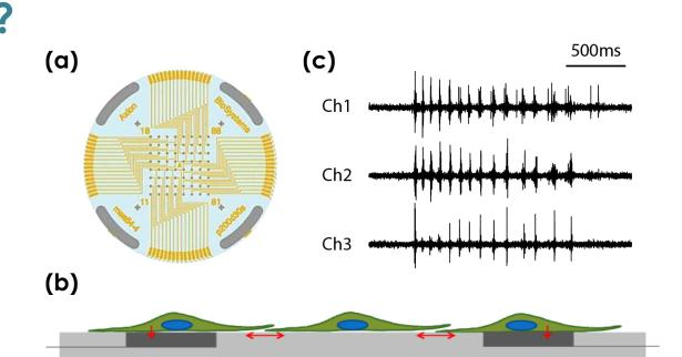
A planar grid of microelectrodes (a) interfaces with cultured neurons or cardiomyocytes (b), modeling complex, human systems over an electrode array. Electrodes detect changes in raw voltage (c) through recording of extracellular field potential.
